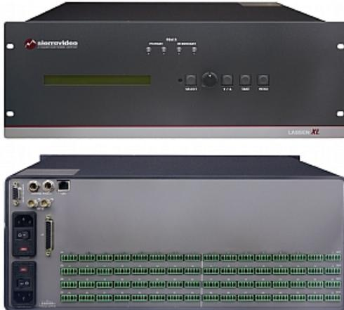
The Lassen XL Series offers flexibility and adaptability to any application where saving space and costs are important. 3232SR-XL is a 32x32 analog balanced stereo audio matrix switcher with redundant power, available in a compact 4RU frame. It offers control via the front panel or remotely via RS-232 or Ethernet
