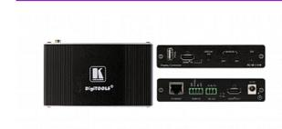
FC-18 is a display ON/OFF controller for 4K@60Hz (4:4:4) HDR HDMI signals. It accepts and outputs an HDMI signal after reclocking and equalizing. On detection of the onset of an input signal FC-18 sends an ON command to the display or projector and on detection of the loss of the input signal FC-18 sends an OFF command. FC-18 can also be used to control a display device manually via front panel buttons, Ethernet or contact closure switches
