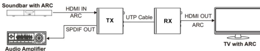
**Scene 5:** Set the Extender to eARC Mode. Then switch the LOOP OUT/AUDIO ONLY switch to right, the HDMI OUT port of the transmitter is set to AUDIO ONLY.
