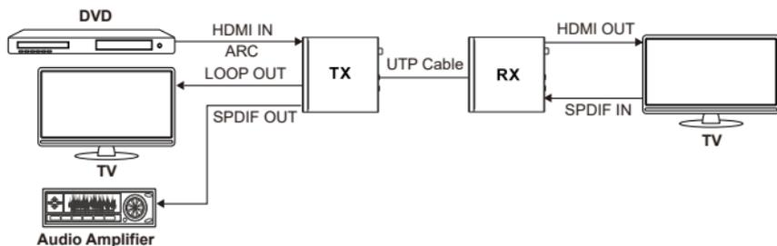
**Scene 3:** Set the Extender to ARC Mode. Then switch the LOOP OUT/AUDIO ONLY switch to right, the HDMI OUT port of the transmitter is set to AUDIO ONLY.
