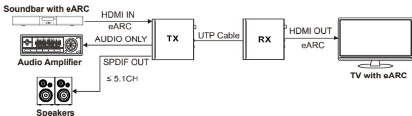
**Scene 6:** Set the Extender to eARC Mode. Then switch the LOOP OUT/AUDIO ONLY switch to left, the HDMI OUT port of the transmitter is set to LOOP OUT.
