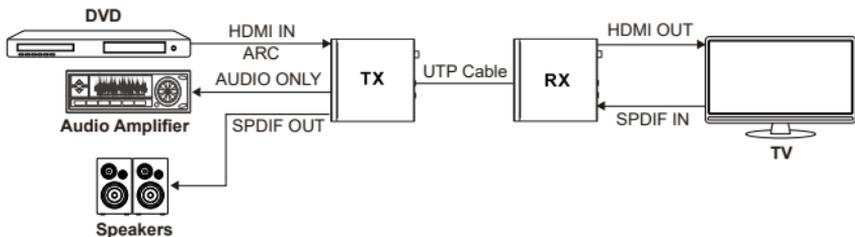
**Scene 2:** Set the Extender to SPDIF Mode. Then switch the LOOP OUT/AUDIO ONLY switch to left, the HDMI OUT port of the transmitter is set to LOOP OUT.
