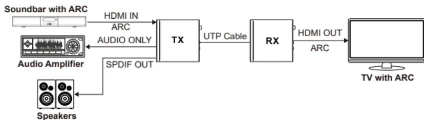
**Scene 4:** Set the Extender to ARC Mode. Then switch the LOOP OUT/AUDIO ONLY switch to left, the HDMI OUT port of the transmitter is set to LOOP OUT.
