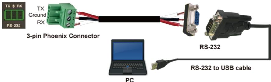
Then, open a Serial Command tool on PC to send ASCII commands to control the product.
